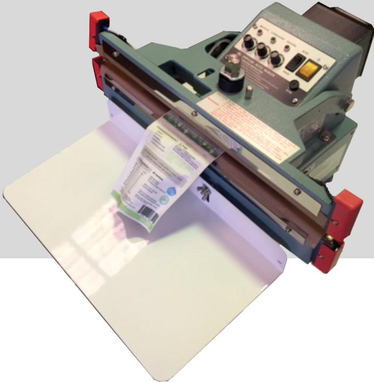
The Innoseal P-450 is a pulse sealer, meaning the element is only energised while the seal jaws are closed. To operate you simply press a switch to close the jaws & engage the sealing it will release automatically.
