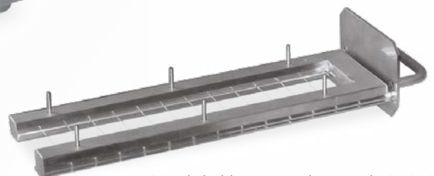
Sample holder in accordance with ISO 3795
