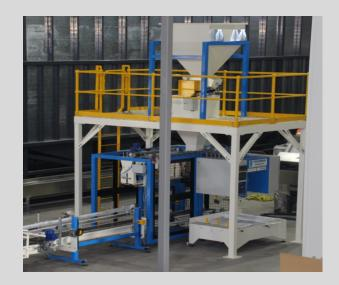
In this system the bags are automatically loaded from the bag magazine to the bag clamp, where the product is placed in the bag. The bag is then transferred from the bag clamp to the bag closing system. This machine will handle gusseted & non gusseted bags but the gussets will not be reformed.
