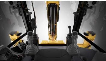
The 444F2 is fitted with pilot controls providing low effort operation, with the ability to switch between ISO (Excavator) or SAE (Backhoe) control patterns with the press of a button. Providing easy and safe operation for operators of any experience or ability.
