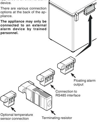
When connecting several appliances via the RS485 interface, the terminating resistor must remain on the last appliance.
