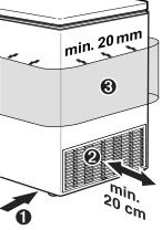
③ Do not place any objects immediately next to the outer housing of the appliance. There must be a gap of at least 20 mm all round in order to ensure adequate heat discharge.
