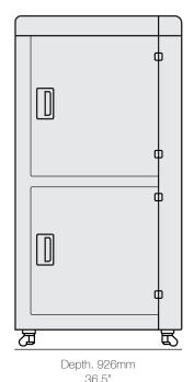
External dimensions 1544 x 926 x 2137mm (WxDxH) 60.8 x 36.5 x 84.1" 635ka Weight Build volume 695 x 385 x 1200mm dimensions (WxDxH) 27.3 x 15.2 x 47.2" LCD screen 8K Resolution 7680 x 4320 pixels Print layer thickness 50-350µm Compatible with Daylight resins 3.3kW in average, 5.5kW Power consumption at peak Light output intensity 1.6 mW/cm<sup>2</sup> Light output wavelength Power input 32A 230v Single Phase Plug type 3 pin IEC60309 Warranty 12 months
