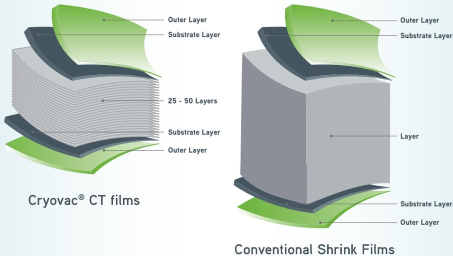
Cryovac® CT series of films provides a radical new technological capability within the packaging industry. This patented innovation incorporates up to 50 discrete micro-layers compared to conventional shrink films, which are typically comprised of 1, 3 or 5 layers.
