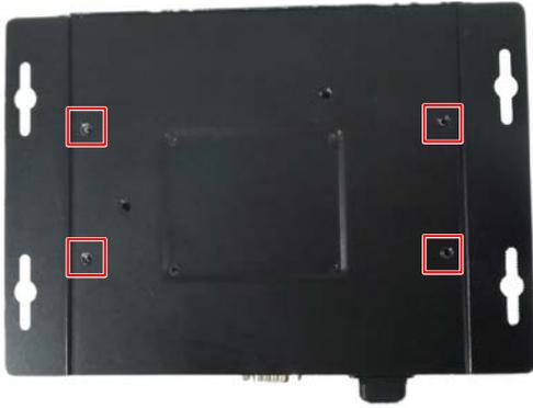
3. Turn the bottom cover to the other side. Place an 2.5" SATA SSD onto the inner side of the bottom cover, align the SSD screw holes, and then use the supplied 4 screws to screw the SSD to the bottom cover from the outside of the bottom cover.
