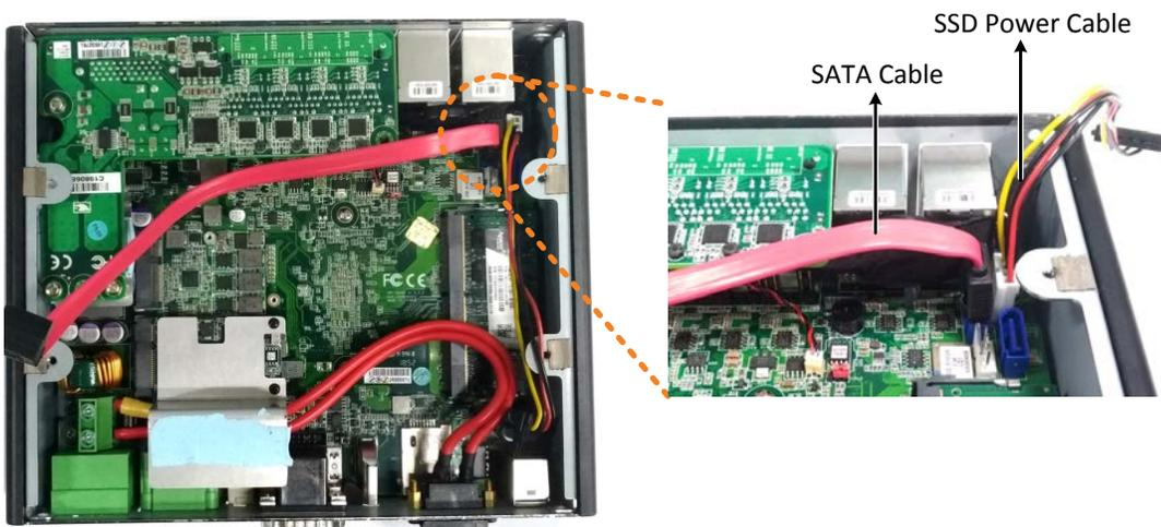
5. Connect the other end of the SATA cable and SSD power cable to the SSD.
