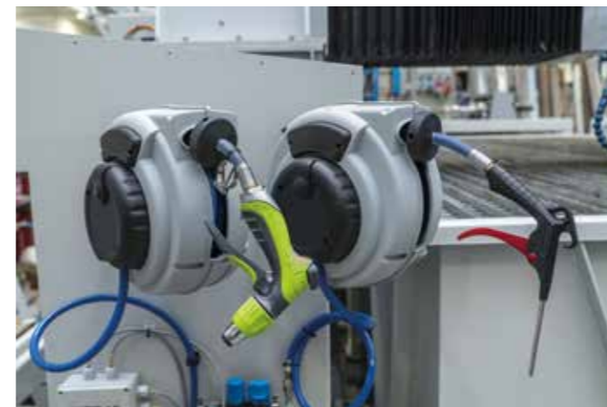
AUTOMATIC HOSE REEL Air and water sprayer kit to clean table and material after the cut. (opt)
