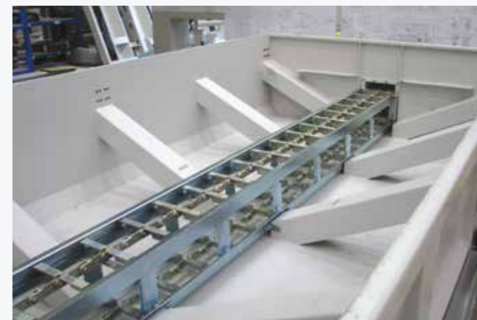
Dredging system for "no maintenance" abrasive removal. The removal system inside the tank is protected both by baskets for collecting scraps and by a metal cage. The tank is ready to install a dredge system for the abrasive removal (opt)
