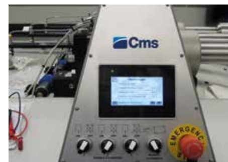
Software-based electronic control of cutting pressure
