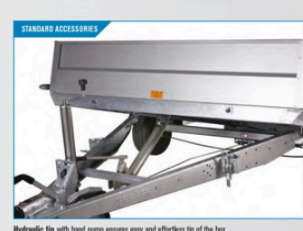
Hydraulic tip with hand pump ensures easy and effortless tip of the box. Powerful fasteners and jockey wheels is standard.
