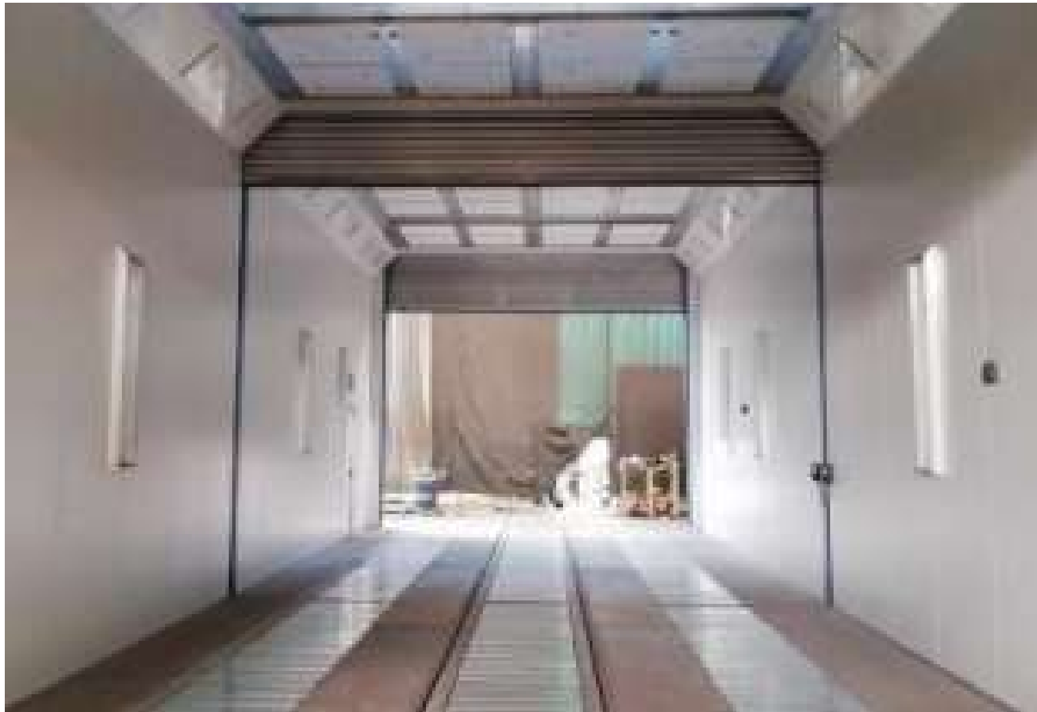
Separating roll-up door to subdivide the booth into two booth parts of equal length
