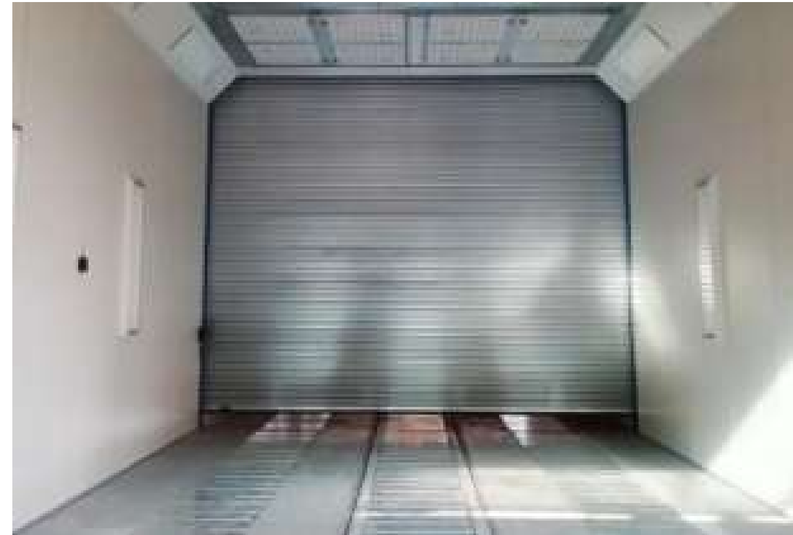
Separating roll-up door to subdivide the booth into two booth parts of equal length
