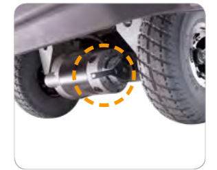
Manual switching lever This lever enables to switch to manual drive at narrow spaces or while battery is discharging.
