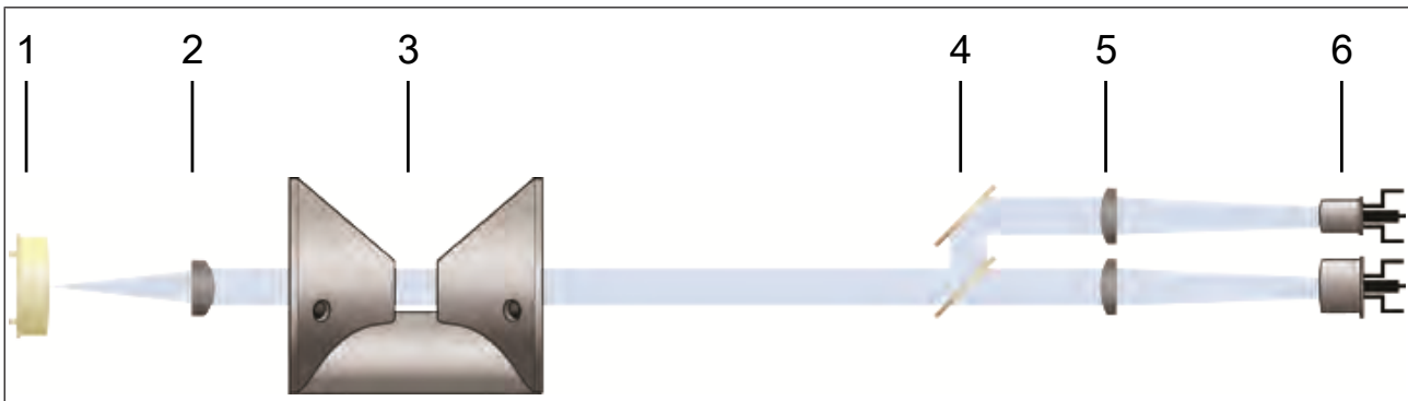
Fig. 12: Operating principle SAC254 Sensor
