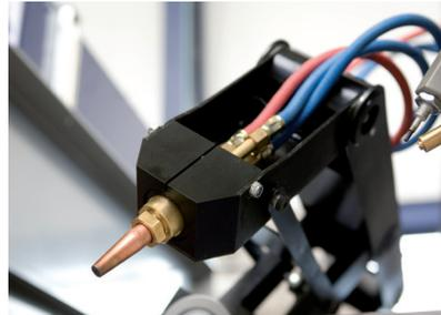
A compact pantograph cutting arm enables the ProCutter 600 to perform 3D cutting routines highly accurate with both plasma and/or oxy-fuel cutting processes.
