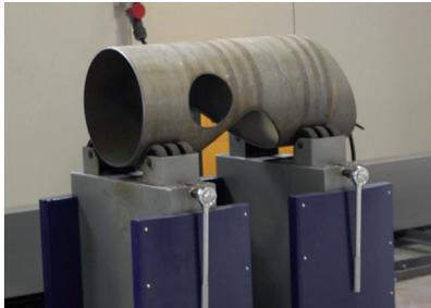
The ProCutter is equipped with adjustable pipe supports to level the pipe at cut location. Furthermore, the ProCutter can be equipped with a rollerball gutter that provides permanent horizontal support.
