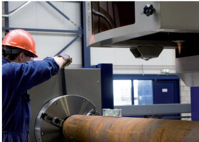
The self centering three jaw chuck is one of the factors influencing accuracy. It achieves high accuracy by clamping pipes securely, avoiding slip and creep (longitudinal movement) during rotation.
