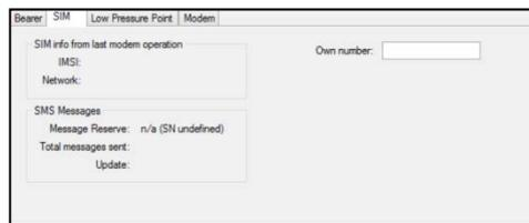
5. *Own Number* should be set to the telephone number of the SIM fitted inside the Cello. This is necessary for both SMS and GPRS operation. If using international format then prefix with "+", e.g. "+44 ..."
