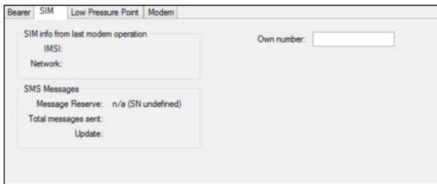
5. *Own Number* should be set to the telephone number of the SIM. This is necessary for both SMS and GPRS operation. If using international format then prefix with "+", e.g. "+44 ..."
