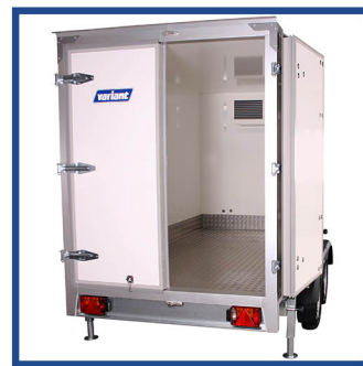
Refrigeration Trailer 2017 K3 Internal: 295x159x192cm External: 442x210x248cm Total Weight: 2,000 kg Payload: 1,300 kg
