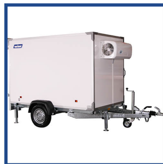
Freezer Trailer 2017 F3 Internal: 289x153x183cm External: 442x210x248cm Total Weight: 2,000 kg Payload: 1,240 kg
