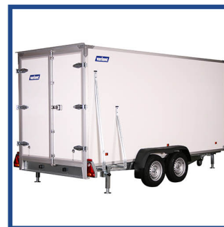
Freezer Trailer 2719 F4 Internal: 404x171x183cm External: 602x234x248cm Total Weight: 2,700 kg Payload: 1,610 kg
