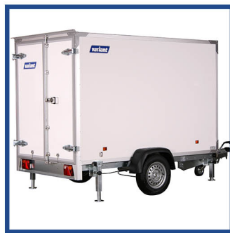
Refrigeration Trailer 1315 K2 Internal: 250x139x162cm External: 393x191x223cm Total Weight: 1,350 kg Payload: 910 kg
