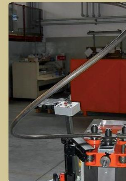
Special tooling to roll handrail
