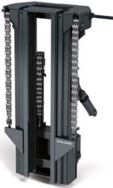
Triplex, 3-stage with freelif
