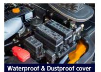
Newly developed Waterproof and Dustproof fuse box and relay box for ease of maintenance.
