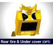
The rear tire cover and under cover with PE material protect the engine, radiator, and components from dusts caused by ground. Also, these options can be selected separately.
