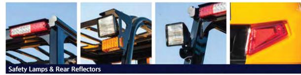
Halogen headlights and rear LED combination lights offer the driver visibility in all circumstances. Rear reflectors mounted on the counterweight enhance safety for the driver and the application.
