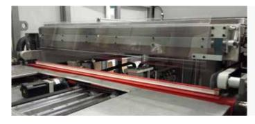
Sheet cleaning system with ionized air: eliminates electrostatic charges from each sheet and from the pallet installed in the loading zone. The utmost in terms of thermoforming quality and safety.
