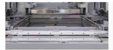
Automatic clamp frame: fully automatic adjustment system with telescopic crossbars. Guarantees cover to all the measurements without the need for manual set up, constantly guaranteeing maximum grip on the sheet
