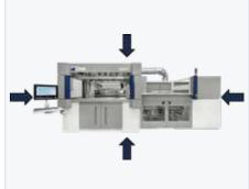
**New machine layout.** Thanks to the new mechanical solutions and closed cabin, the **overall height of the machine** is now **reduced by 25%** compared to previous models.
