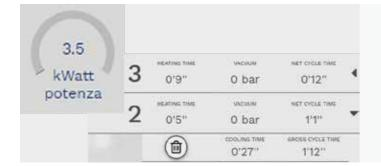
Energy reading system: device for measuring energy with every machine cycle. The energy value is saved in the production control for a quick assessment of the batches produced.
