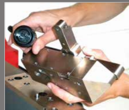
B2: PRE-ALIGNED LOWER TOOL HOLDERS Alignment pins allow for changeover to any other standard Haeger tool holder without alignment verification
