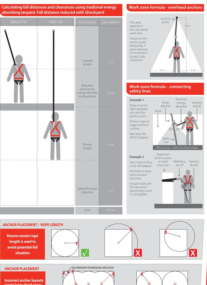
Incorrect anchor layouts create large dead zones. Correct anchor layouts reduce dead zones
