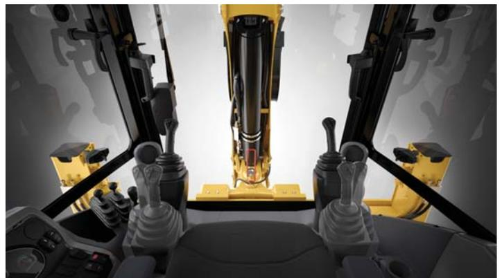
The 444F2 is fitted with pilot controls providing low effort operation, with the ability to switch between ISO (Excavator) or SAE (Backhoe) control patterns with the press of a button. Providing easy and safe operation for operators of any experience or ability.
