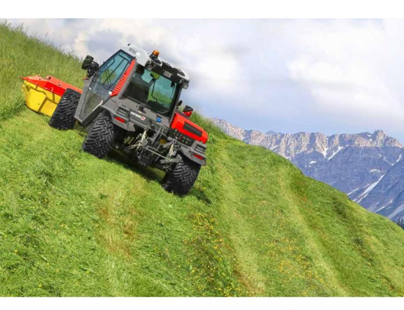
The intelligent 4 wheel steering system of the new Metrac allows 5 steering modes: front, rear, 4 wheel and crab steering as well as offset 4 wheel steering.
