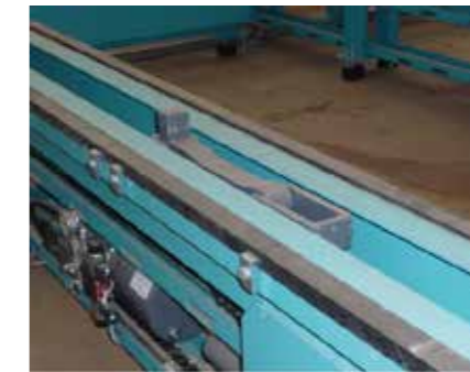
Cross-conveyor with lifting pins for conveyance in two directions.
