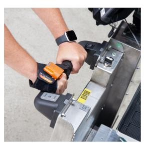
NoBa Solution slowed down the speed of TENTE's E-Drive system to 5 km/h. This way, even if a worker bumps into the trolley up front, the trolley will stop automatically without causing any injuries. A foot protection in front of the castors also prevents potential accidents.
