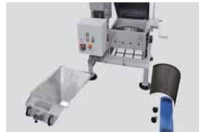
Due to the Quick snap fasteners used on the GSL series machines, the machines can be opened for cleaning and maintenance quickly without the need for special tools.
