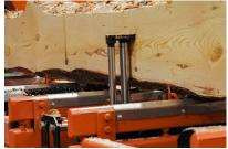
Two independently powered taper rollers help to optimize log yield.
