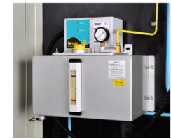
▲ Auto Lubrication System
