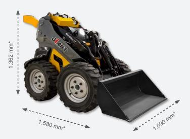
\*Dimensions measured on standard tyres, without attachment and with folded drivers platform.
