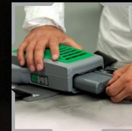
Sealed inside the unit during operation, the long-life lithium-ion battery is protected from moisture when decontaminating and will not disconnect or bump off while operating.
