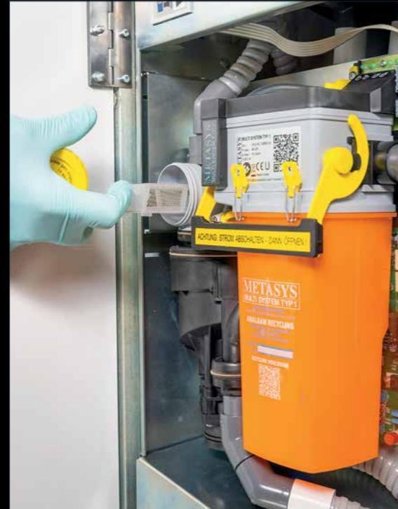
The integrated Metasys MST1 amalgam separator is easily accessible for cleaning and maintenance.
