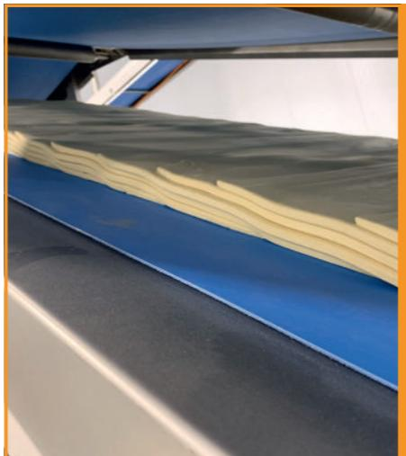
The Rijkaart continuous folding system has been designed so that the supply conveyor is situated just above the outfeed conveyor. The reduced drop height minimizes the stretching of the dough as it is transferred from one conveyor to the other, thereby maintaining the integrity of the fat band encapsulated within the dough sheet. Alternatively, with the cut-and-stack method, the dough sheet is cut to length and then penny-stacked onto a conveyor mounted below the retracting unit.
