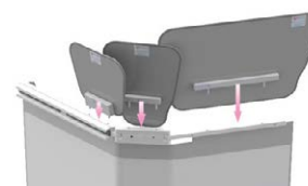
Slot into docking holes
