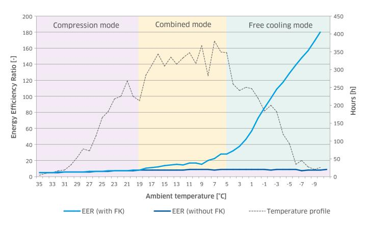
Calculation example for a QUANTUM chilled water set
