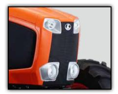
**Quad Front Lamps** Two main head lights at the bottom and two work lights on the top of front mask increase visibility especially in dark and inclement conditions.
