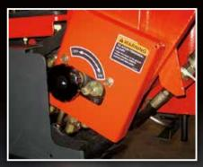
Kubota Shockless Ride (KSR) The KSR helps to minimize fatigue by "smoothing out" the ride of the tractor. This feature is particularly useful when your tasks include a lot of tight turns or lifting and dumping of heavy loads. It makes handling round bales far less jarring.
