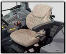
**Deluxe Air-ride Seat** All Grand X tractors are equipped with a reclining and automatic height and weight control Air-ride seat that's especially designed to absorb shock and reduce operator fatigue.
