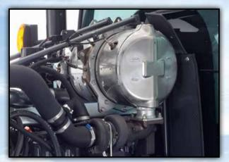
**Diesel Particulate Filter (DPF) Muffler**
