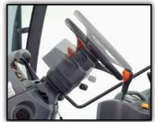
**Tilt and Telescopic Power Steering** Tilt and telescopic steering offers the ideal driving position while power steering makes steering easier even in rough terrain.
