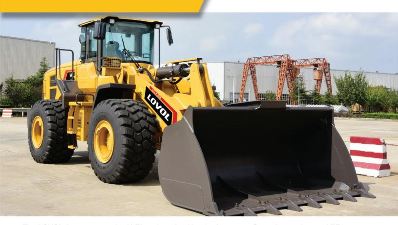
The LOVOL 7 tonne capacity ALFA series wheel loader features a Cummins engine, and ZF power-shift transmission. It also has Pilot oil operated joysticks. 4 wheel disc brakes, as well as a Luxury lined and fully sealed A/C cab. This machine has limited electrically controlled functions, eliminating many of the problematic items!
