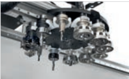
Revolver magazine with 12 overhead positions and 12 on the X carriage, reducing cycle times to the minimum.
