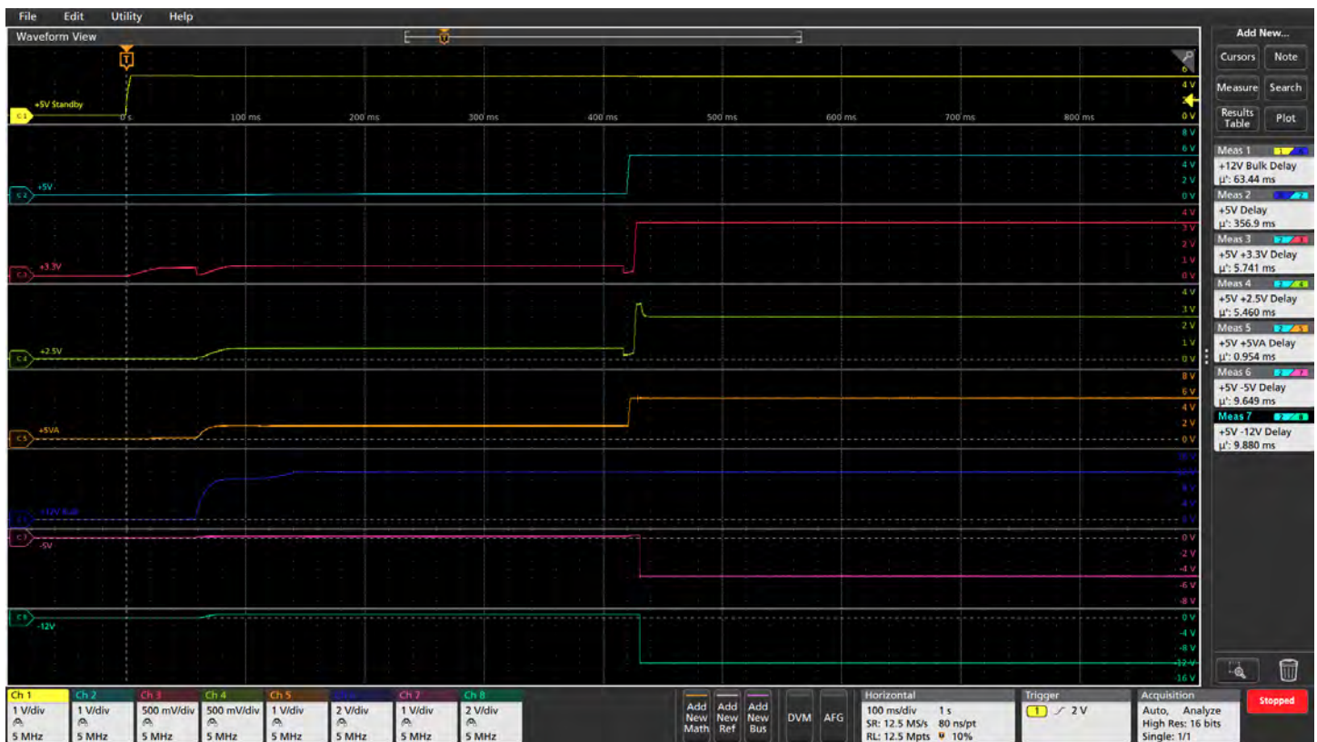
Using automated measurements to characterize power supply bring up.
