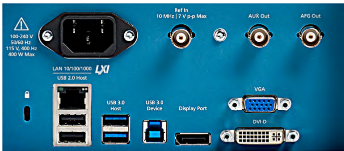
The I/O you need to connect the 5 Series MSO to the rest of your design environment.
