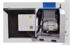
To minimize the needed floor space and make the machine easy to move the control cabinet is integrated into the machines soundproof housing.
