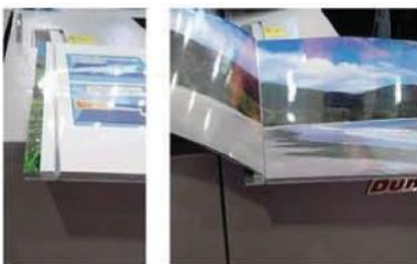
Gap lamination for layflat binding
