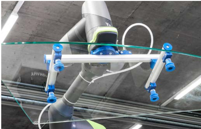
Modular PXT gripper handling a glass pane
