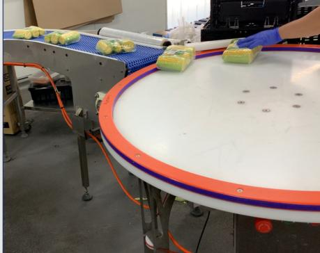
Our rotary accumulation turntable configurations can handle multiple containers sizes and products. The rotary design is flexible and the top discs diameters are 900 mm and 1200 mm.
