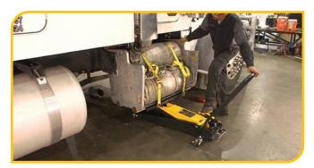
Omega Lift Equipment offers a fast and easy to use DPF Step Housing Handler, that a single technician can operate.
