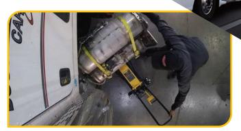
Smooth rolling 360 degree casters allow a single technician to Remove and Reinstall a DPF Step Housing unit, increasing shop manpower efficiency and lowering costs.
