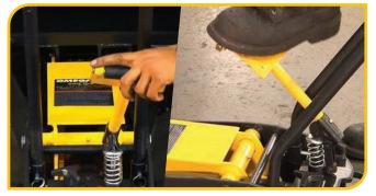
The Pump handle allows the technician to operate the DPF Handler with a hand or foot pump.
