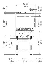
CWII Cold Water inlet 1 CWI2 Cold Water Inlet 2 D Drain
