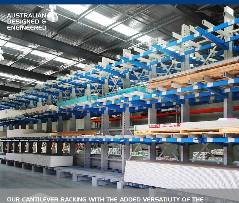
OUR CANTILEVER RACKING WITH THE ADDED VERSATILITY OF THE SPREADER SYSTEM—SPECIALLY DESIGNED TO STORE FLEXIBLE PLASTERBOARD & SHEET PRODUCTS PERFECTLY LEVEL
