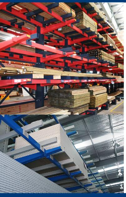
The Emrack Cantilever Spreader System provides leading sheet & plasterboard manufacturers with an ideal solution for the storage and safe handling of plaster and sheet product—along-side palletised & flexible materials.
