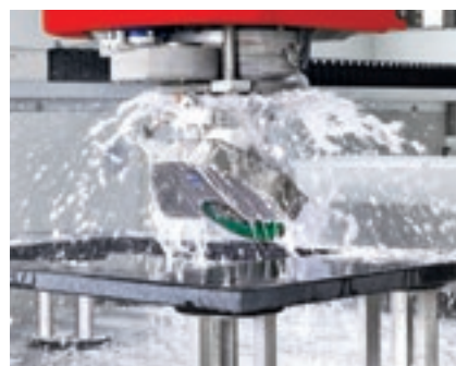
45° disc cuts for joints.
