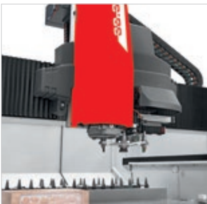
8-position rotary magazine on the head, reducing the time taken to replace the most frequently used tools.
