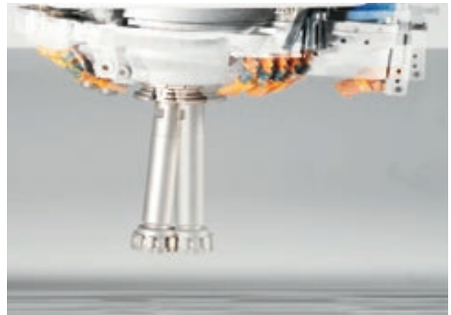
Tilting T axis ( \pm 2.5^\circ ) for making recesses for kitchen tops on the tilted table.
