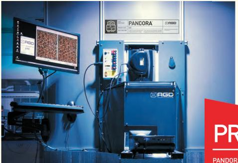
**Pandora**<sup>™</sup> and **Atlas**<sup>™</sup> are bespoke sets of test equipment designed and developed by AGD Systems. They are dedicated to the testing of the 640 digital vision pedestrian wait area detector and 100% of units manufactured at AGD are Certified by Pandora and Atlas.
