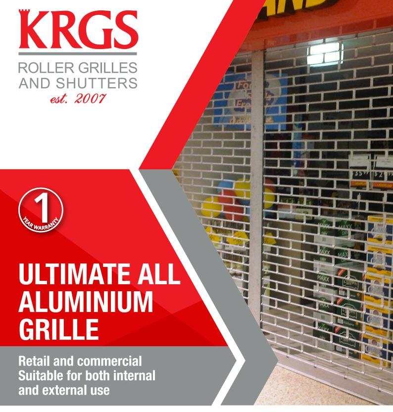
The KRGS All Aluminium Grille has a sleek, easy to operate curtain manufactured from 12mm aluminium extrusion tubing connected with a 22mm wide aluminium extruded links creating a symmetrical, brick like pattern. The KRGS All Aluminium Grille allows retailers to retain visual product branding and airflow while their products are secure.
