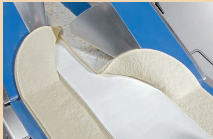
A homogeneous dough band and a consistent layer of fat are the basis for the high quality of the dough band.
