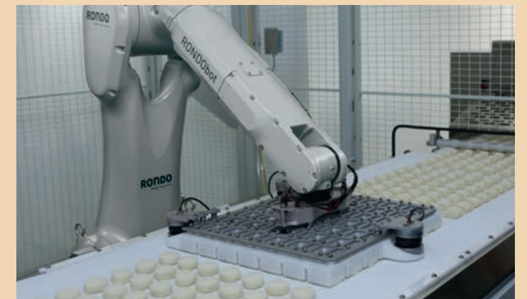
RONDObot is a rounding tool to mould high hydrated square dough pieces into round artisanal breads and buns.
