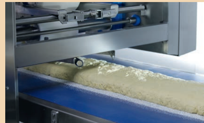
With the MIDOS dough-band former, you achieve the desired dough structure.
