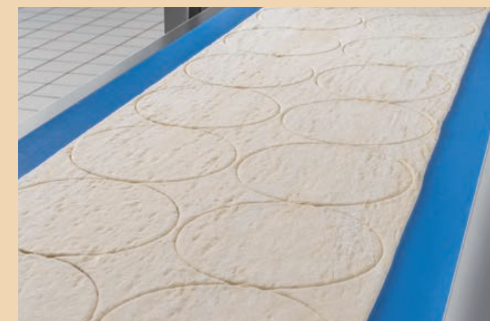
A dough band without stress is the requirement in order that pizzas stay round.
