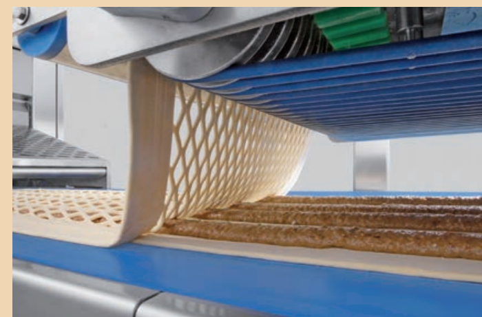
With sandwiching, you cover the filling with a second dough band and then stamp out the products.
