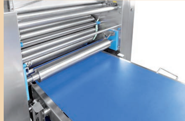
The wide-opening protective covers, the belt management system and the free spaces between the individual line components ensure good accessibility to all points where cleaning is required.
