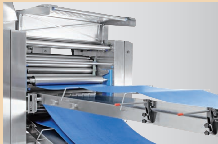
Only materials that can be easily cleaned are used. The conveyor belt also has sealed edges.
