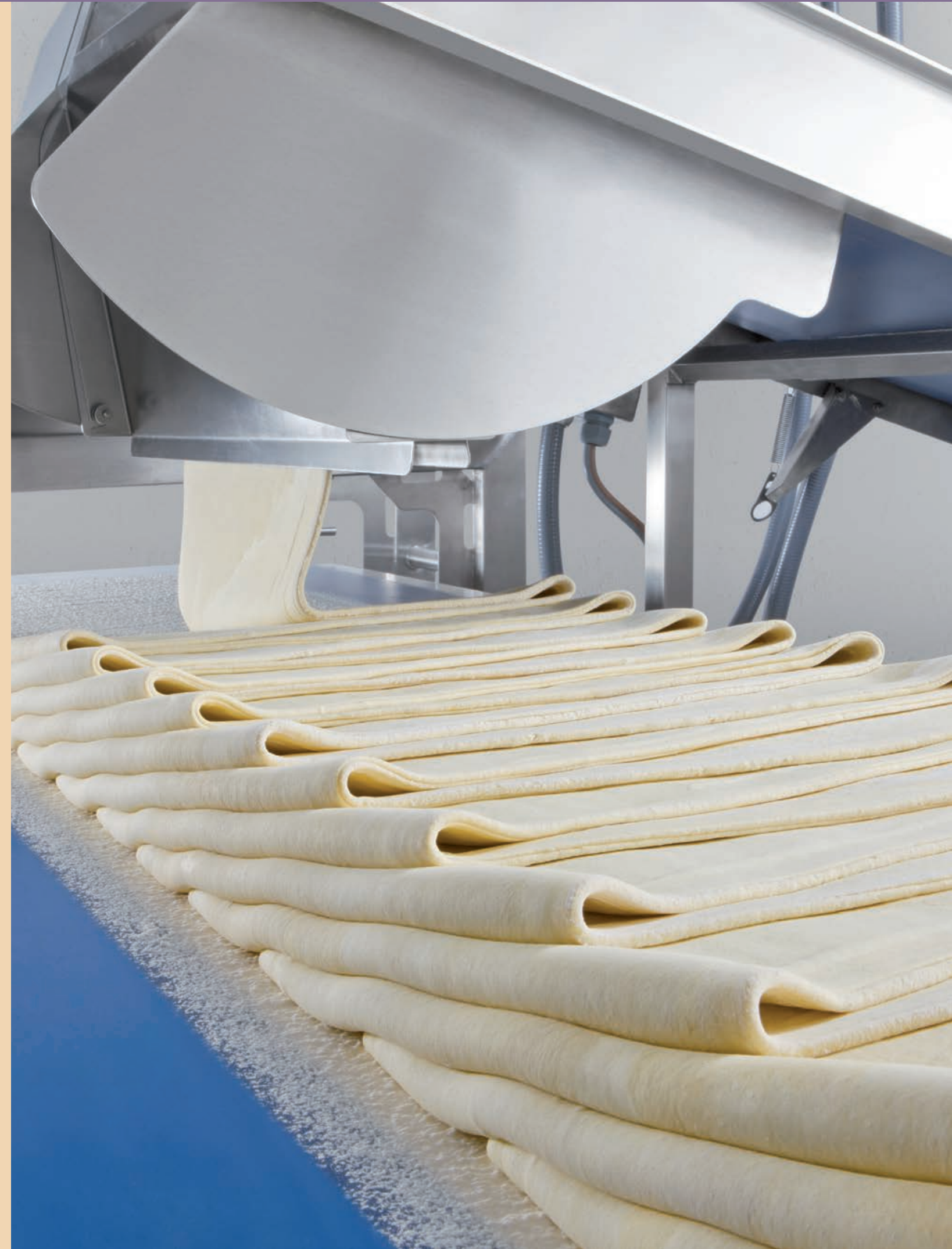
Large satellite heads with two lower rollers treat the dough band particularly gently.
