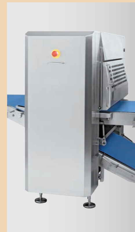
The thinnest dough bands can be produced with special calibrating devices.
