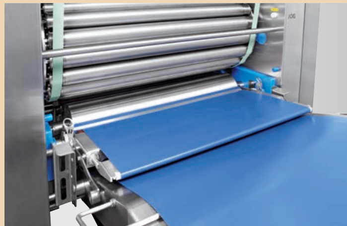
Large satellite heads with two lower rollers treat the dough band particularly gently.
